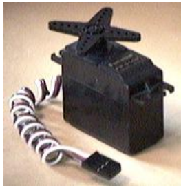
Figure 7. Servo motor FP-S148
