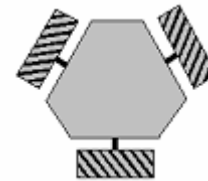
Figure 15. Three omni-directional wheel drive system [12]
