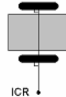
Figure 14. Two-wheel differential drive system [12]
